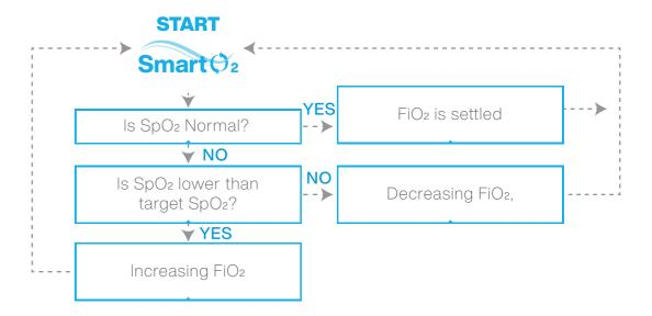
By comparing SpO<sub>2</sub> concentrations measured from patients within the range of FiO<sub>2</sub> prescribed by clinicians with the target SpO<sub>2</sub>, it automatically adjusts FiO<sub>2</sub> depending on SpO<sub>2</sub> to provide oxygen to patients and prevent hypoxia or hyperoxia.
